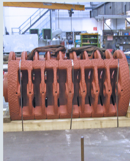
Rotor after refurbishment
